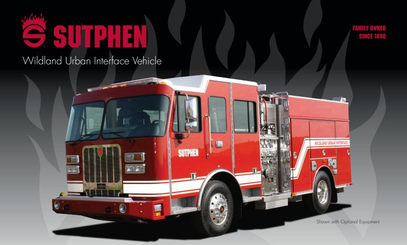
Sutphen Wildland units are the perfect mix of form and function. These trucks are designed with a short overall length, and un-matched angles of approach and departure exceeding 20 degrees. This special attention to chassis design allows them to operate in the roughest of terrain, or on a busy highway. Capability for stationary high-volume pumping or pump and roll, you'll be ready for any size situation.
