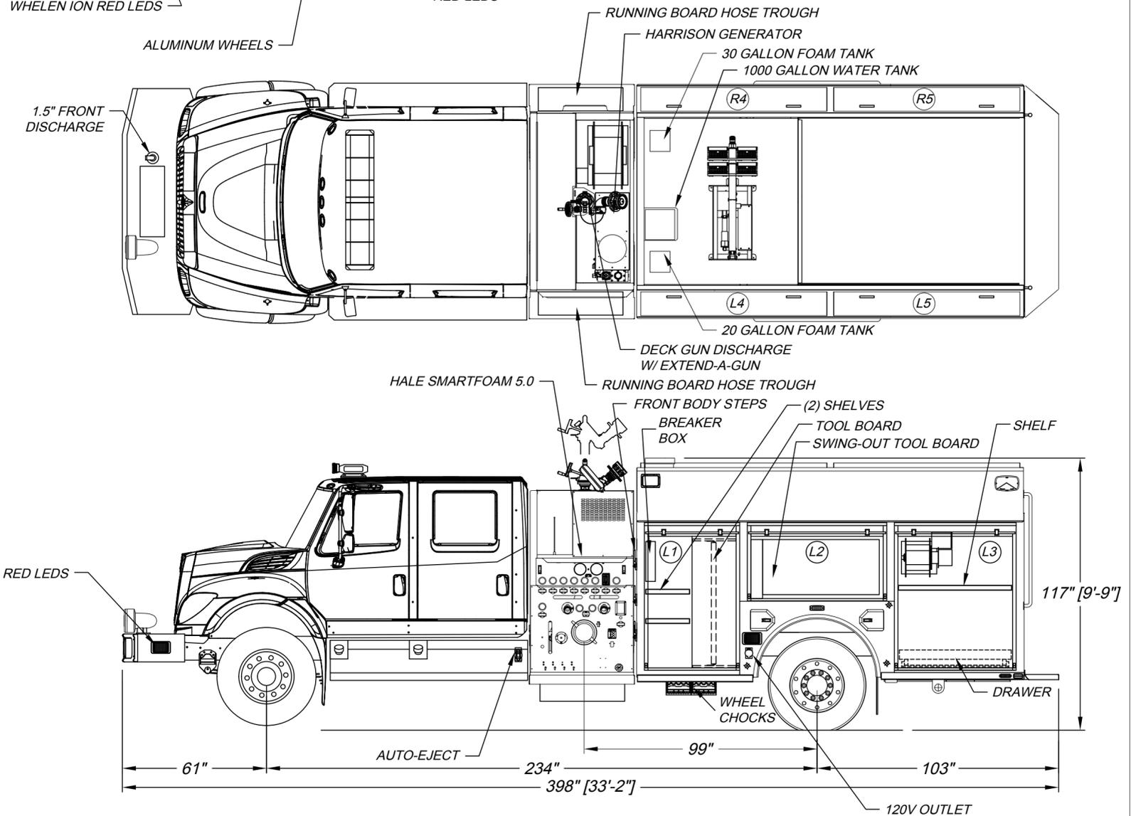
DIMENSIONS SHOWN ON THIS DRAWING ARE APPROXIMATE AND ARE SUBJECT TO MINOR DEVIATIONS DURING CONSTRUCTION.
