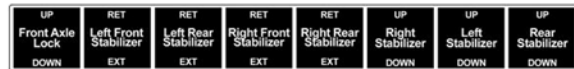
Sutphen Tag 406-A IC Label P/N 3001035-0001 Manual Override Outrigger Controls Label 50% Scale
