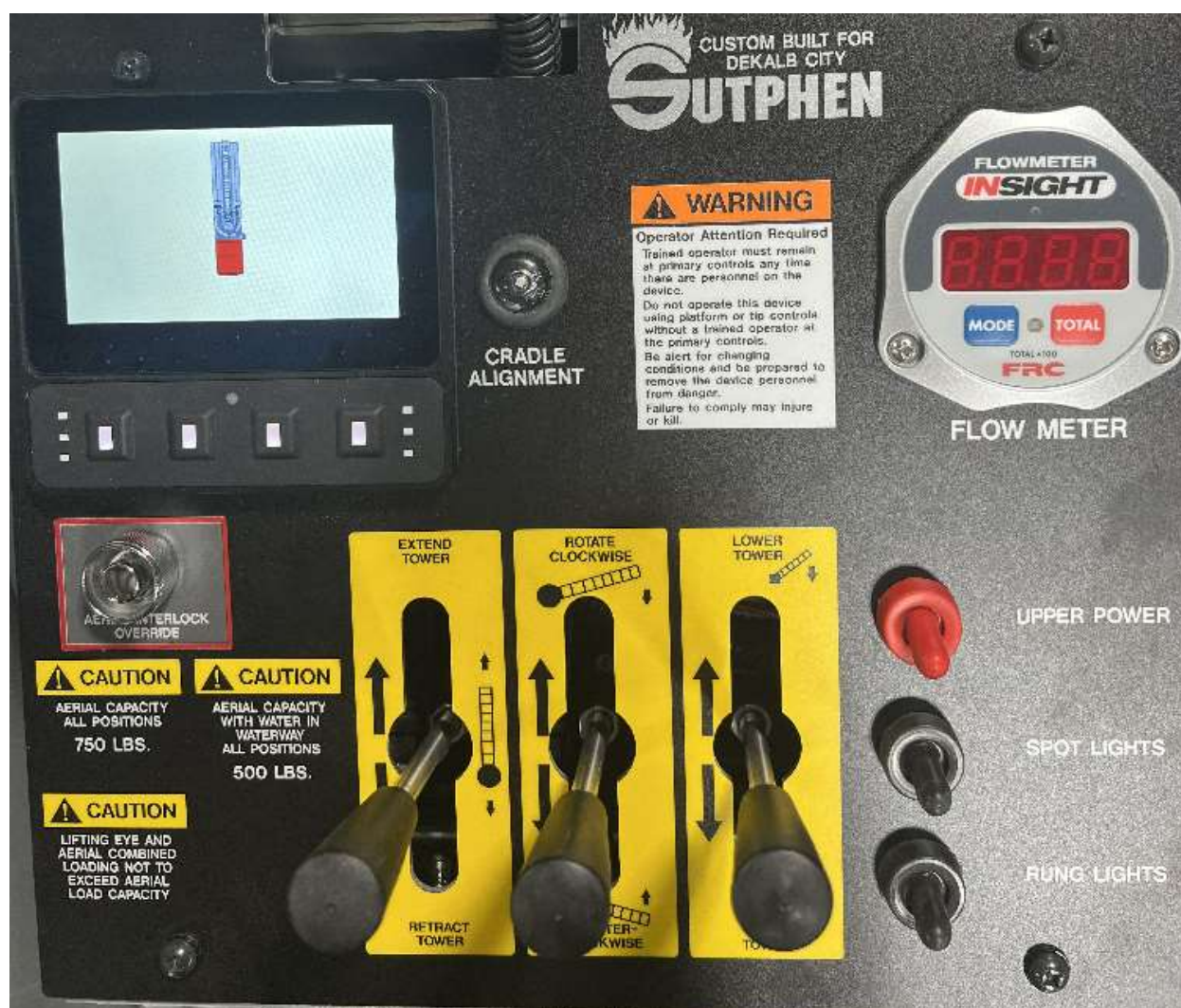
Figure 3- Ladder Controls At Pedestal
