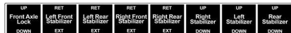
Sutphen Tag 406-A IC Label P/N 3001035-0001 Manual Override Outrigger Controls Label 50% Scale
