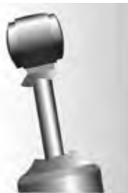
Damaged dust cover and / or shock body
