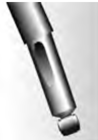
Bent or dented shock absorber
