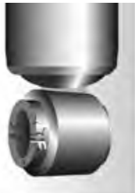
Damaged upper or lower bushing
