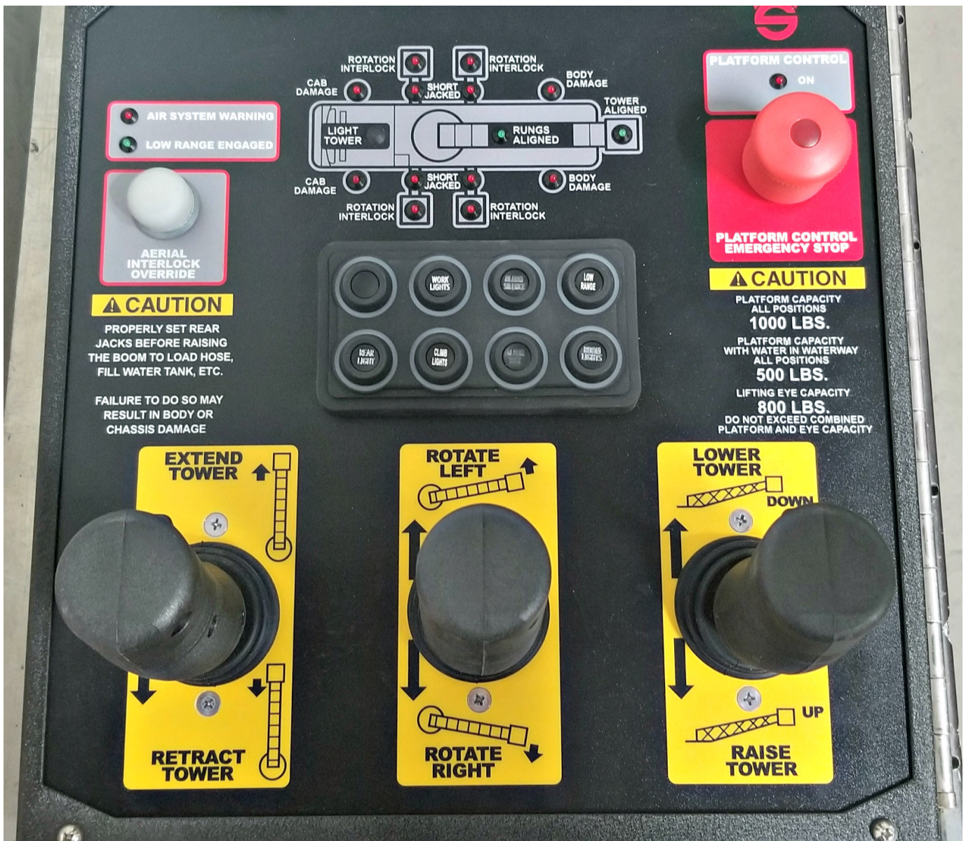
Pedestal Control Panel
