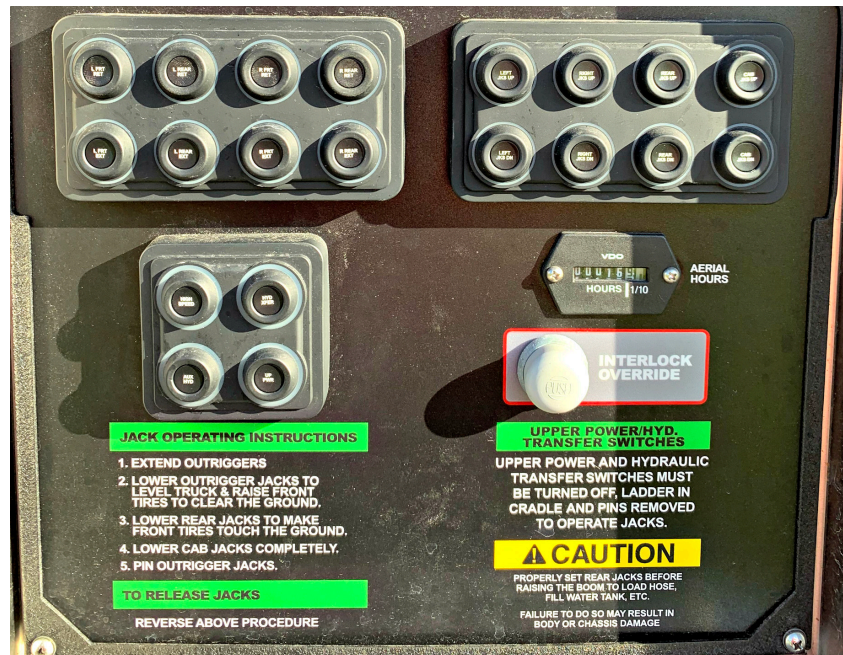
Jack Control Panel
