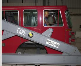
• Sutphen meets or exceeds all ECE R29, SAE J2422, and SAE J2420 Cab Crash Test standards, as well as FMVSS 207 and 201 Seat Belt Pull Tests.
